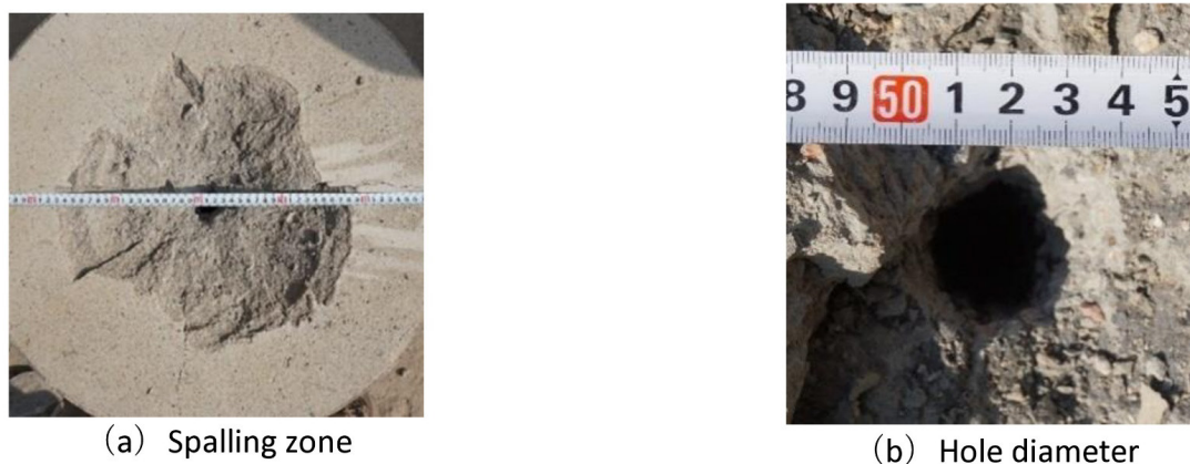
Figure 4. Jet penetration experiment results on plain concrete.
