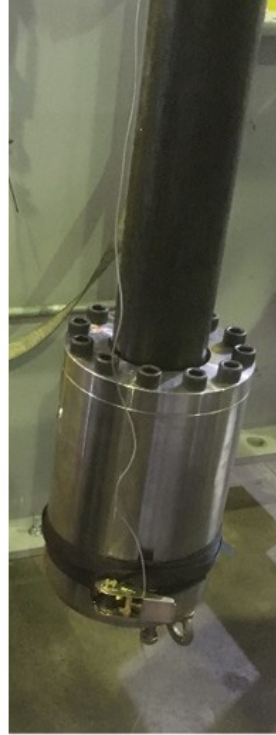
Figure 3 Detail of stainless-steel connector mounted at the free end of the umbilical cable sample. Courtesy of STRESSTEC Engenharia.
