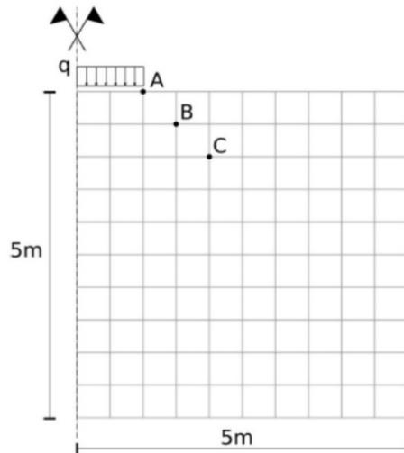
**Figure 3** Strip footing of a saturated granular material, coarsest mesh of 10x10 FE
