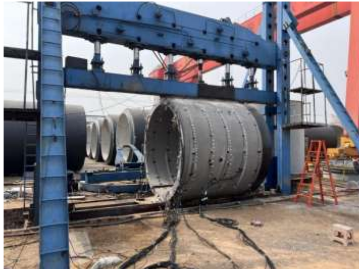
Figure 4 Three-edge bearing test method device.
