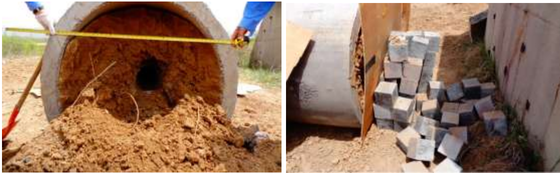
Figure 5 Penetration effect of the \phi 148 mm shaped charge jet on the asphalt/soil/concrete composite target.
