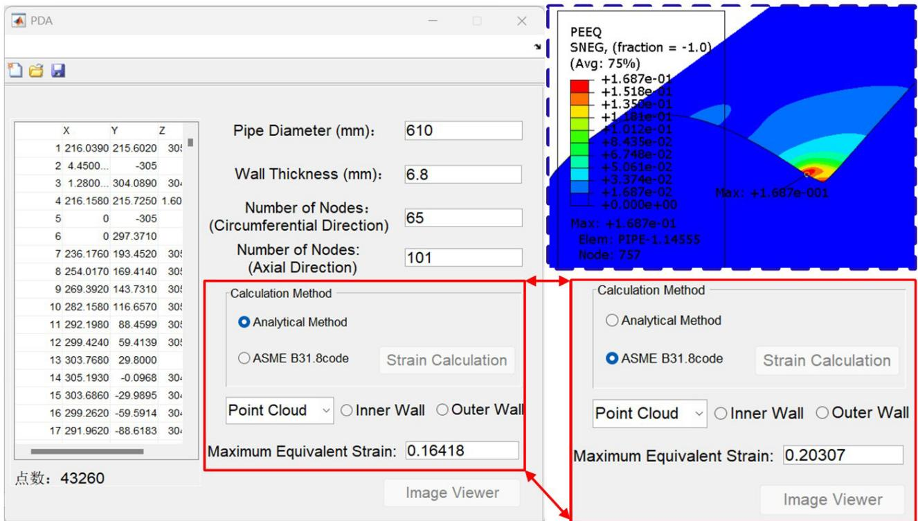
Figure 16. Output interface of dent strain calculation software.
