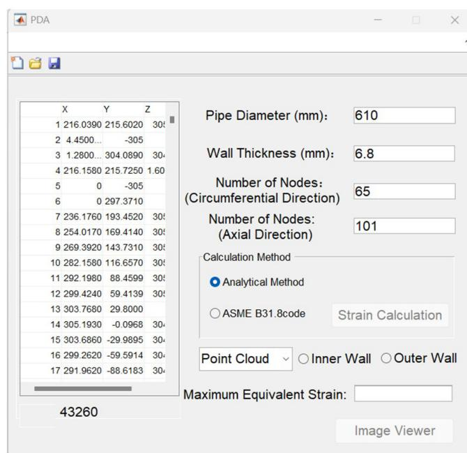
**Figure 15.** Input interface for dent strain calculation software.
