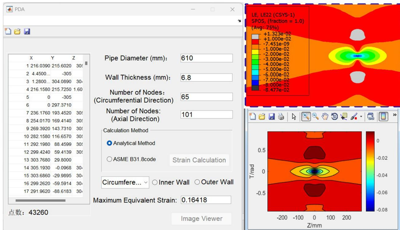
Figure 17. Strain contour plot of the software.
