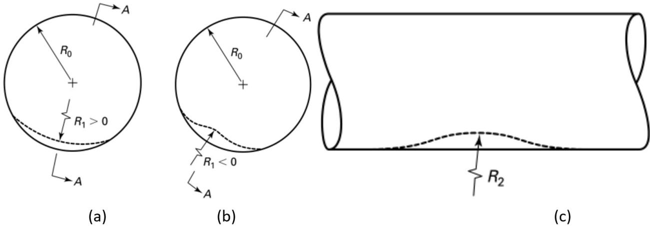
**Figure 6.** Dent strain estimation (ASME B31 Committee, 2018): (a) non-reentrant, (b) reentrant, and (c) longitudinal profile.
