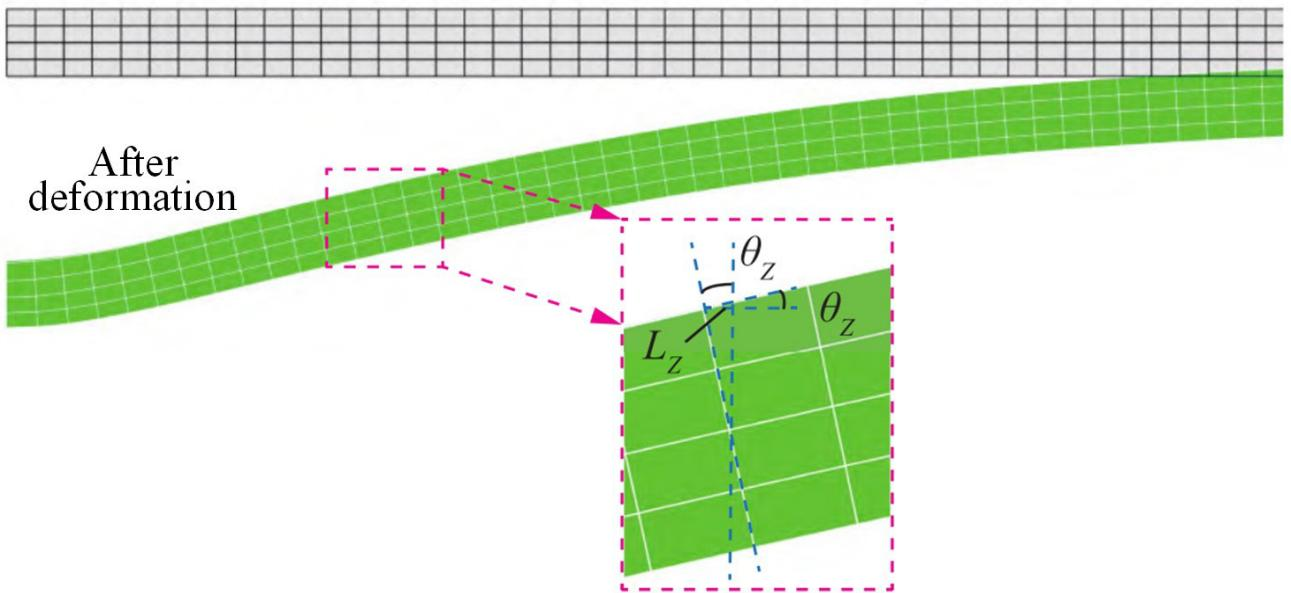
**Figure 5.** Geometric relation of dent points in the axial section of a pipeline before and after deformation.
