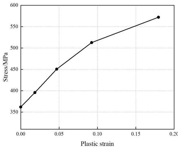
**Figure 14.** True plastic stress-strain curve.
