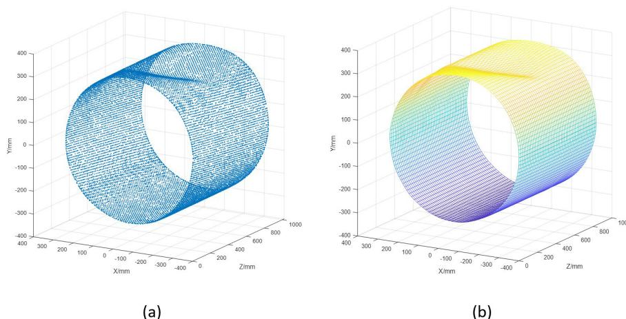
**Figure 2** 3D laser scanning pipeline dent point cloud model regularization processing: (a) point cloud after pretreatment, and (b) regularized mesh.
