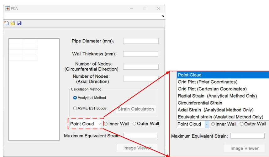
**Figure 13.** Software Interface of dent strain calculation module.
