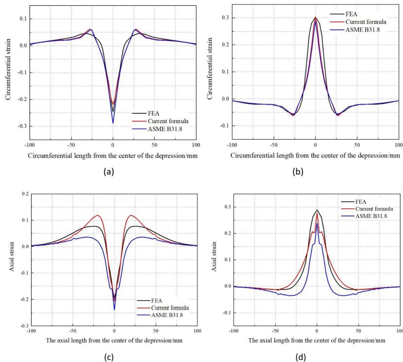
**Figure 11.** Comparison of dent strain results: (a) circumferential strain on the outer wall, (b) circumferential strain on the inner wall, (c) axial strain on the outer wall, and (d) axial strain on the inner wall.
