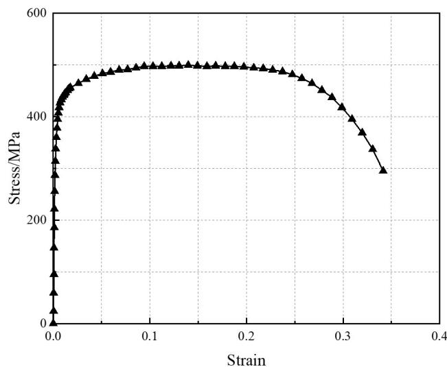
**Figure 7.** Engineering stress-strain curve used in FEA model.
