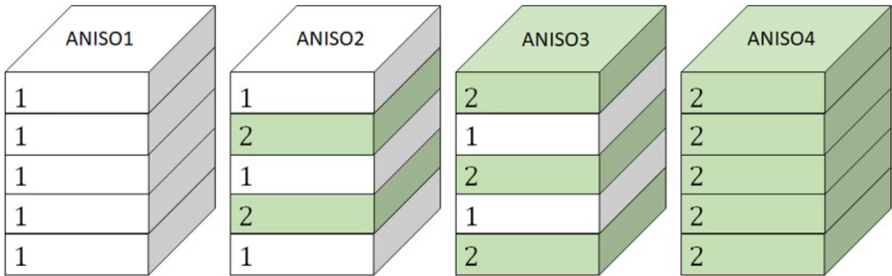
Figure 9 – Plies configurations along the thickness – ANISO1 up to ANISO4
