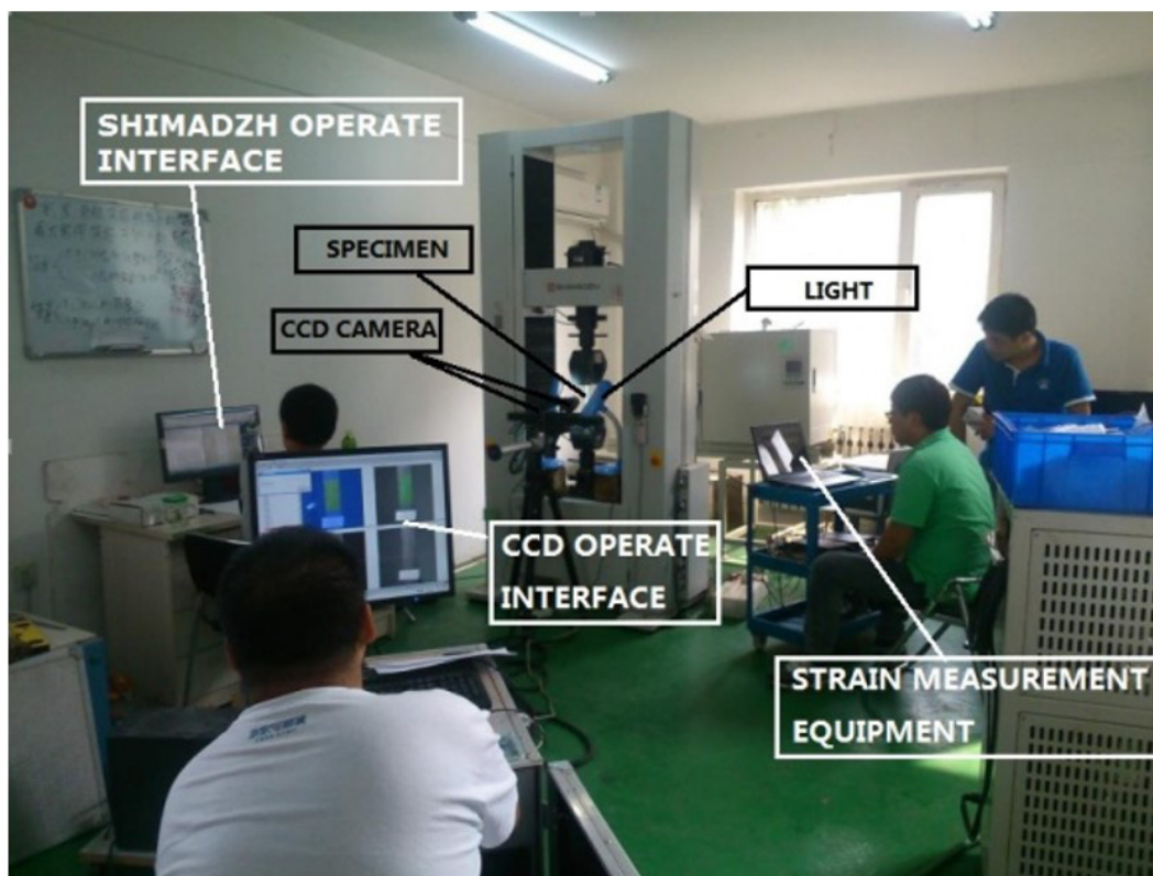
Figure 3 Test of GLARE laminates under tensile loading.
