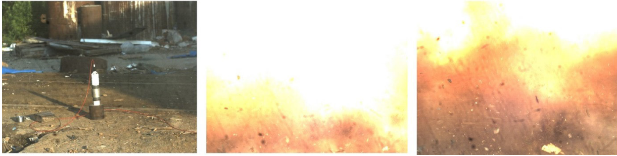
Fig. 8 High speed camera shows detonation of JH-2 target explosive covered with 10mm casing with input v^2d value of 68\text{mm}^3/\mu\text{sec}^2 .
