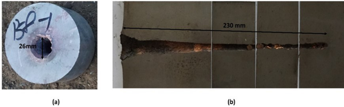
Fig. 11 Penetration behavior of shaped charge jet into steel target (a) diameter (b) depth of penetration
