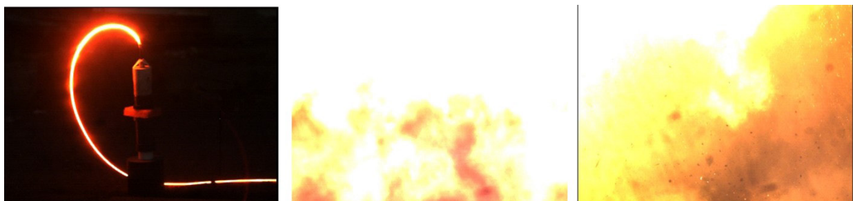
Fig. 7 High speed camera shows detonation of JH-2 target explosive covered with 20mm casing with input v^2d value of 68 \text{mm}^3/\mu\text{sec}^2 .
