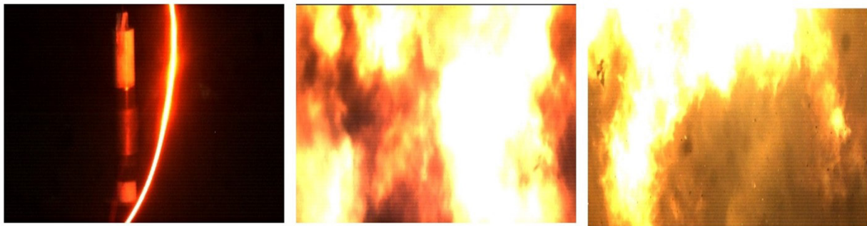
Fig. 9 A high-speed camera records JH-2 explosive detonation using buffer plates (10mm steel, 60mm aluminum), replicating a 40mm grenade's performance against 10mm steel cover for JH-2 explosive.
