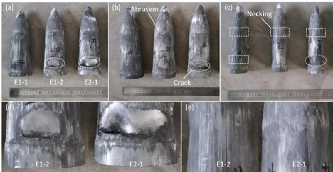
Figure 8 Photographs of the recovered ECDPs: (a) front view, (b) rear view, (c) side view, (d) Enlarged view of tensile crack, and (e) Enlarged view of necking.
