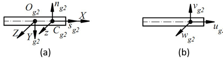
Figure 5 Definitions of (a) Local coordinate system and (b) through-thickness displacement fields in the GFRP laminate 2 section
