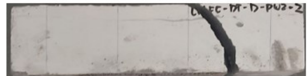
(b) Shear Failure from C-PW2
