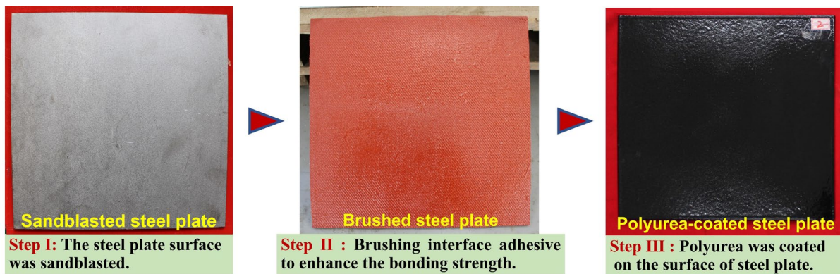
Figure 1 Manufacturing process of the PCSPs.
