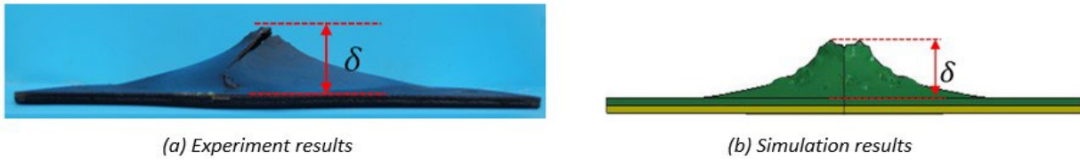
Figure 6 Maximum deformation ( \delta ) in experiments and simulations.
