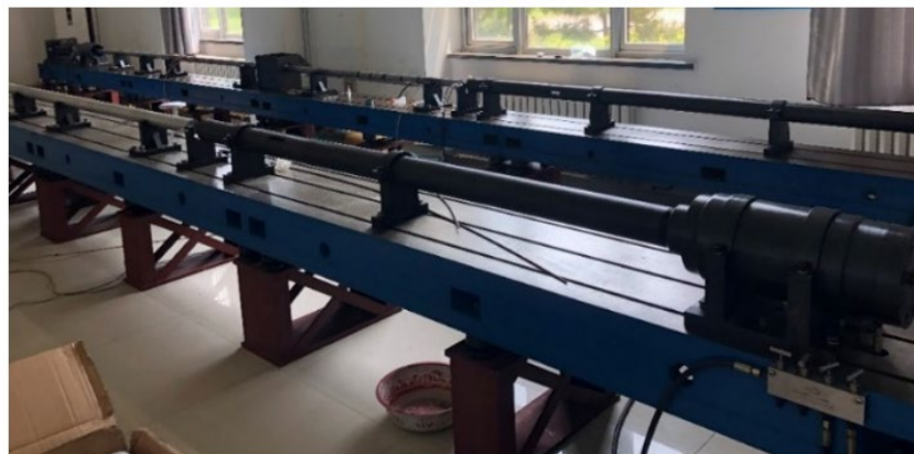
(b) Schematic diagram of SHPB device
