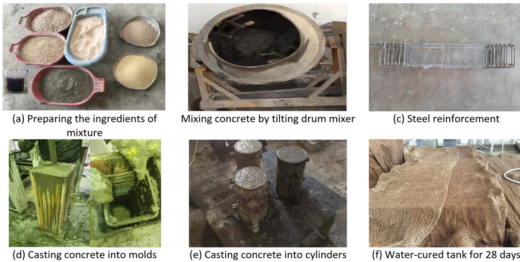
Figure 3 The mixing, casting, and curing of reinforced concrete columns
