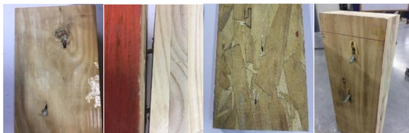
Figure 8. Brittle and premature failure of the self-tapping screws after fatigue at the CLT-LSLs connection.
