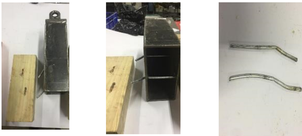
Figure 5. Ductile failure after fatigue of the dowels in the CLT-Steel connection.
