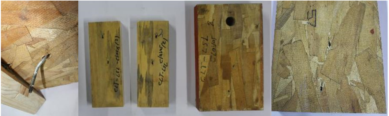
Figure 6. Ductile failure of the nails after fatigue in the CLT-LSL connections.
