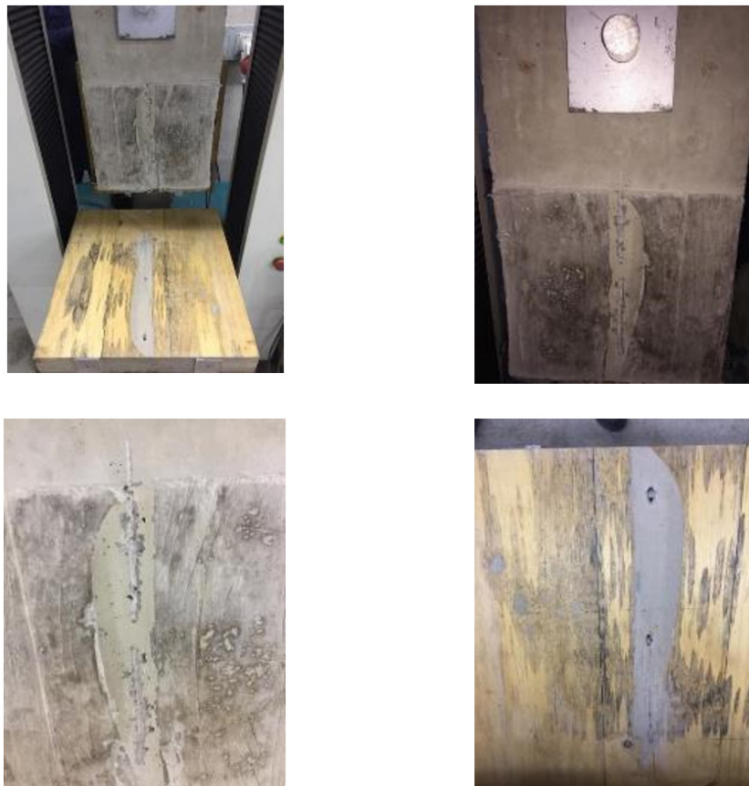
Figure 7. Brittle failure of the CLT-RCwo connection (without posttension bars). The failure was similar to the previous CLT-RCw but not so abrupt which is evidenced by less visible damage at the shear plane in the concrete.
