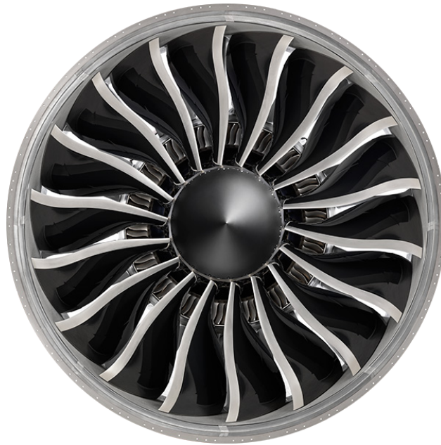
Fig. 1. Carbon-fiber composite fan blades of GENx engine
