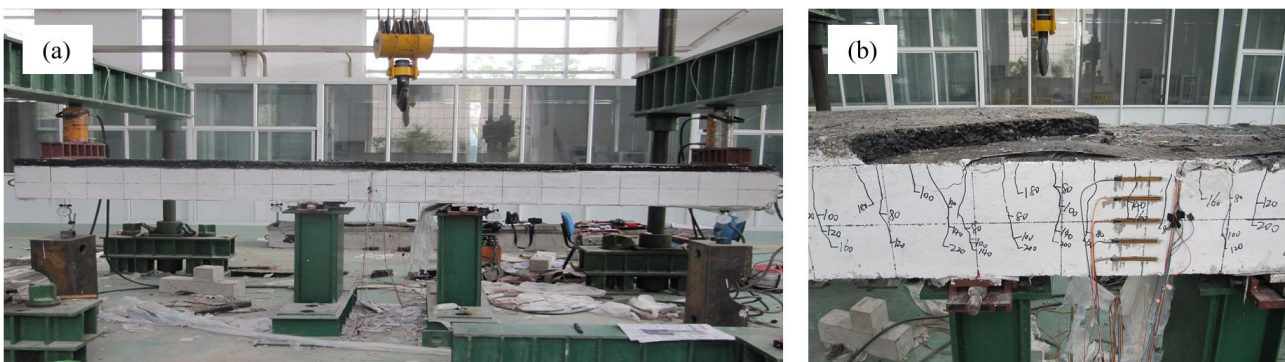
Figure 9 A representative specimen in the test rig: (a) Specimen before the bending test; and (b) Specimen with asphalt layer partially removed after the test.
