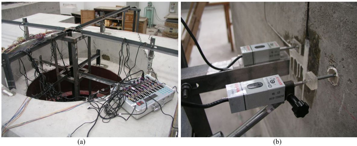
Figure 10: Crack width test of concrete: (a) data collection, (b) measuring gauge.
