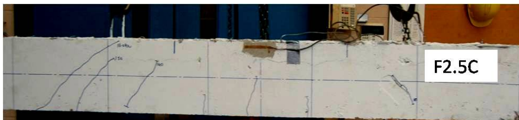
Figure 9: Main shear crack at the other side of pre-crack
