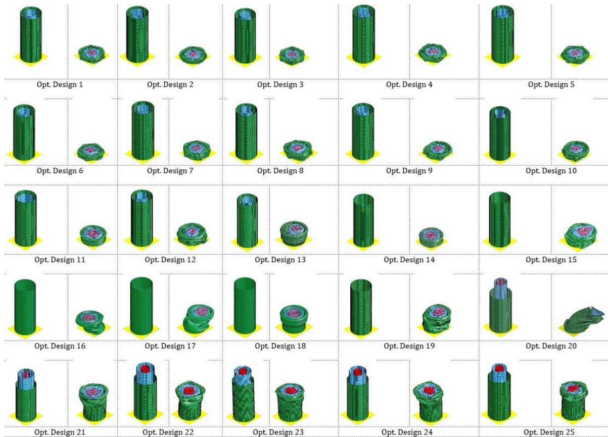
Figure 9: Undeformed and deformed shape of optimum tube systems for different SEA and CFE values
