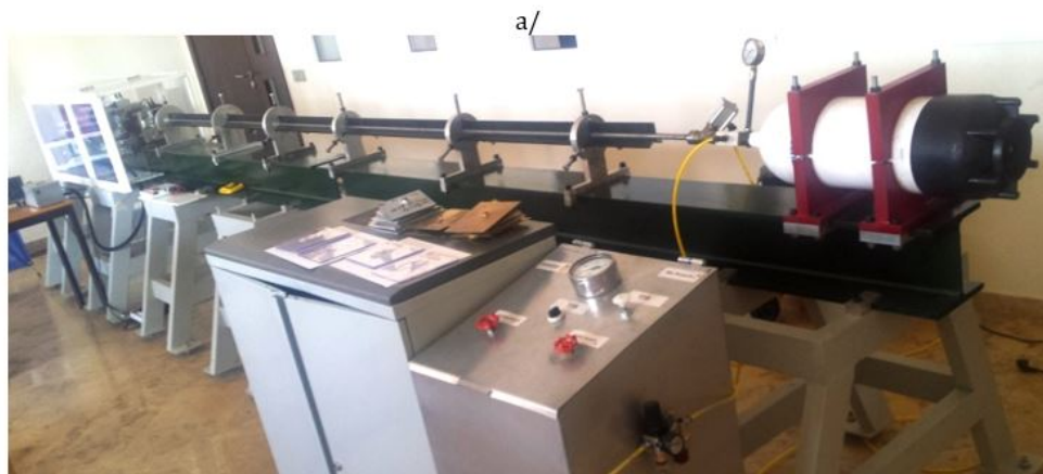
Figure. 1: Gas gun set-up used for perforation tests at high impact velocities and temperatures, a/ general scheme b/ photo of the system with the thermal chamber installed
