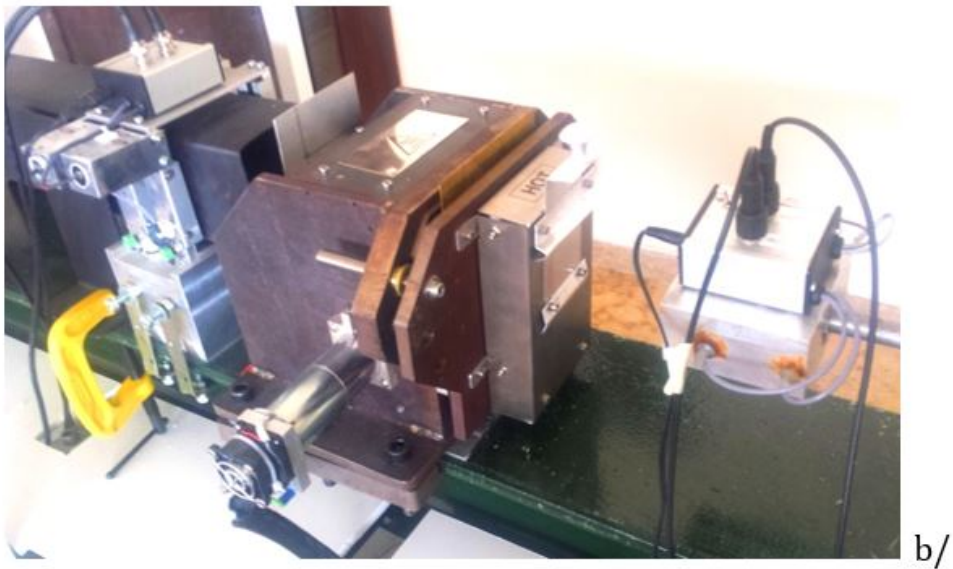
Figure. 3: Thermal chamber for heating up the target plate specimens, a/ schematic representation of the process of air mixing b/ general view of the thermal chamber
