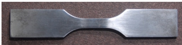
Figure 3: Specimen in the form of a sheet that was used in the stress and fatigue test.
