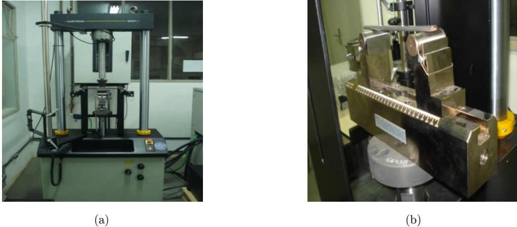
Figure 3: Servo-hydraulic test machine: (a) general view and (b) four points bending fixture (only the bottom part is shown).
