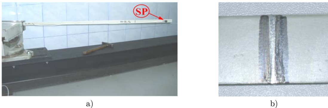
Figure 9: General view of the test stand and magnification of the first step damage
