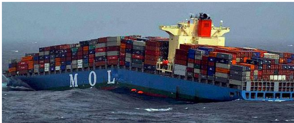
Figure 1: MOL Comfort - 313 m length container ship broke in two in June 2013 (Vesselfinder.com, 2013).
