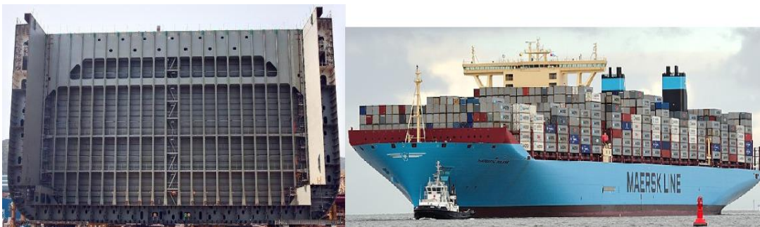
Figure 8: Typical 3,500 TEU double sided - double bottom container ship.
