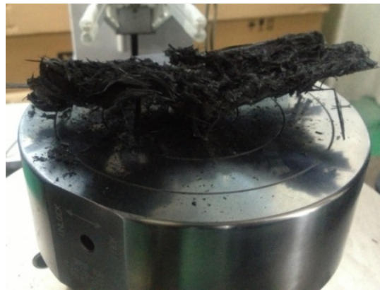
Figure 2: Typical morphology of composite sinusoidal specimen after crush testing.
