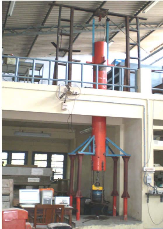
Figure 6 Instrumented drop mass setup.
