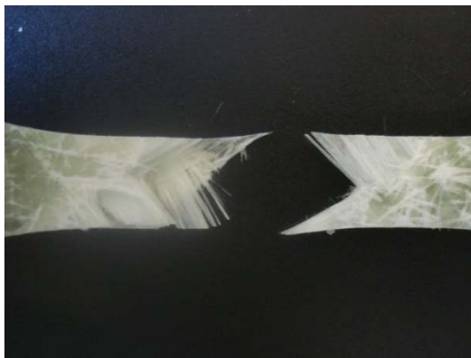
b) Failure of off-axis tests samples , 45^\circ
