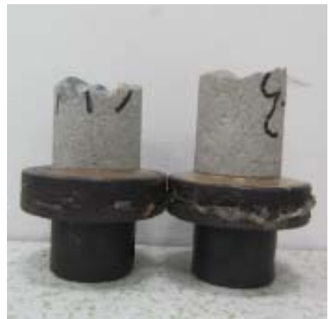
(c) The quasi-static tensile failure pattern
