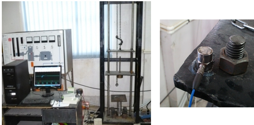
Figure 5: Drop hammer setup and the acceleration sensor.
