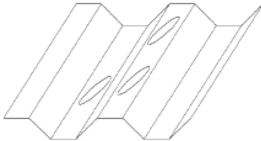
Figure 4: The local buckling form in corrugates of plate.
