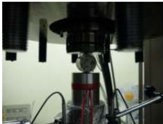
Figure 3: The process of splitting test.
