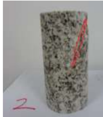
Figure 10: The granite specimen before and after a uniaxial compression test.
