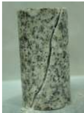
Figure 12: Failure pattern of granite samples under triaxial compression tests.
