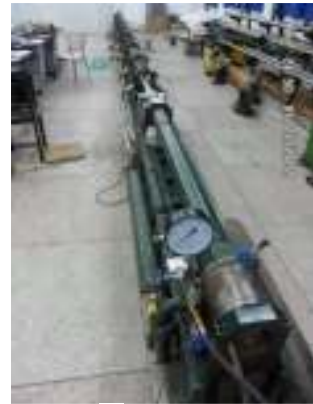
Figure 2: \phi 75 mm SHPB device.
