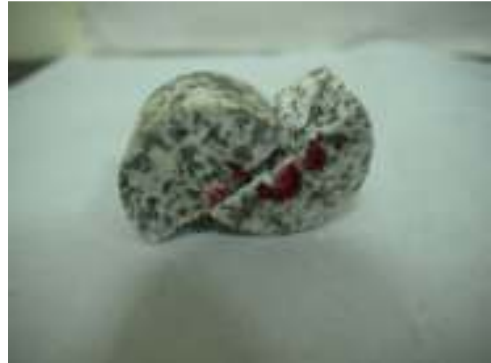
Figure 9: The failure mode of splitting test.
