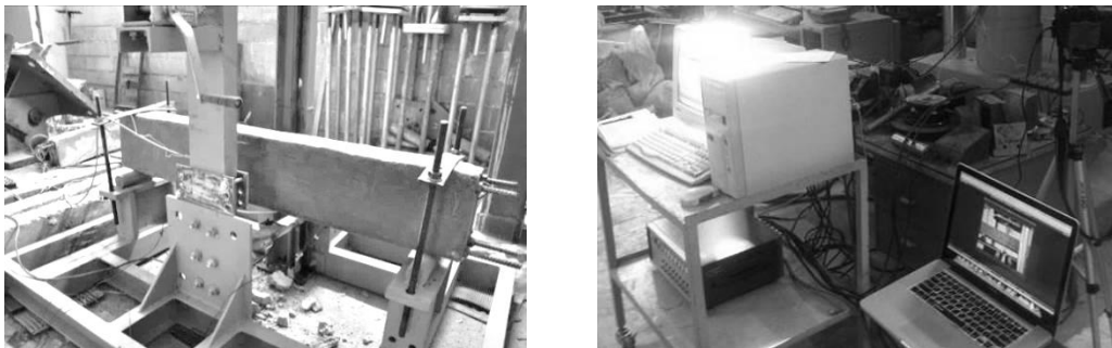
Figure 4: Provided drop-weight test setup, dynamic data logging, and imaging systems.
