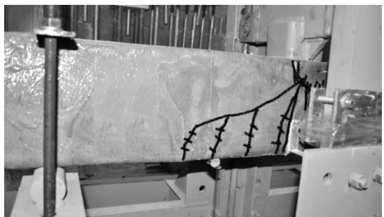
(c) Shear-flexural resin cracking and CFRP rupture raise in CP retrofitted beams
