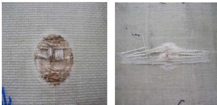
Figure 6: Damage area observed on the impact side and on the non impact side for a 4 layered laminate clamped in the opposite direction.
