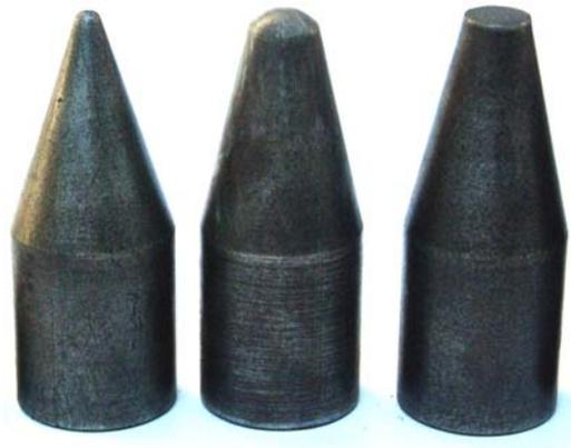
Figure 2: Cylindro-conical projectiles with three different nose geometries
