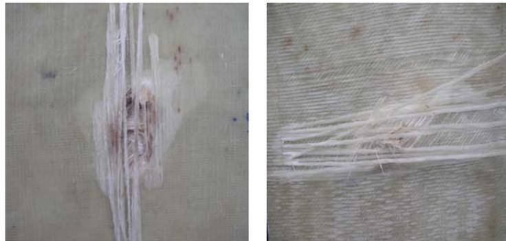
Figure 5: Damage area observed on the impact side and on the non impact side for a 6 layered Anti symmetric thick laminate.
