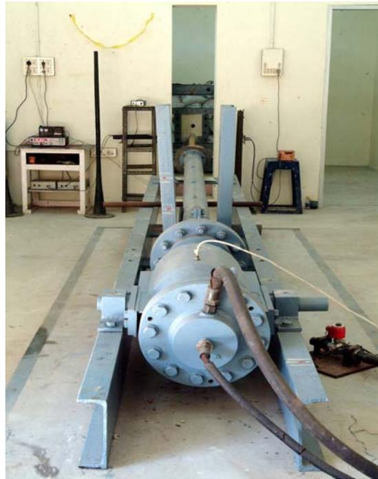
Figure 1: Gas Gun projectile launcher – Experimental setup
