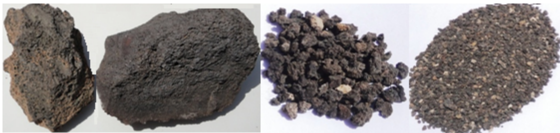
Figure 4 Samples of natural volcanic rocks and aggregates obtained after crushing and sieving
